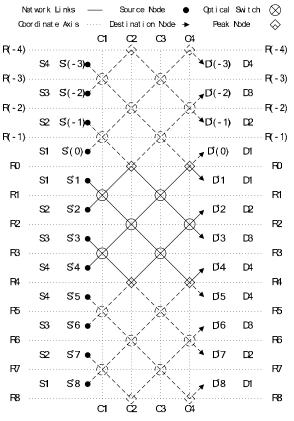
Figure 5. Structure of the Tri-network for a 4×4 WRON
